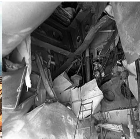
A view looking through the hole in the hull of USS Samuel B Roberts after a mine strike on 14 Apr 88.
