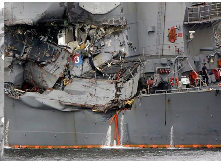
Damage to USS Fitzgerald (DD-62) after a collision with a merchant vessel in 1917.
