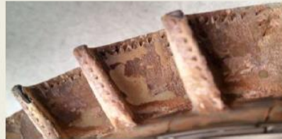
Typical build-up on blade
