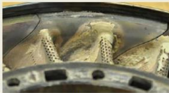
Typical build-up on vane
