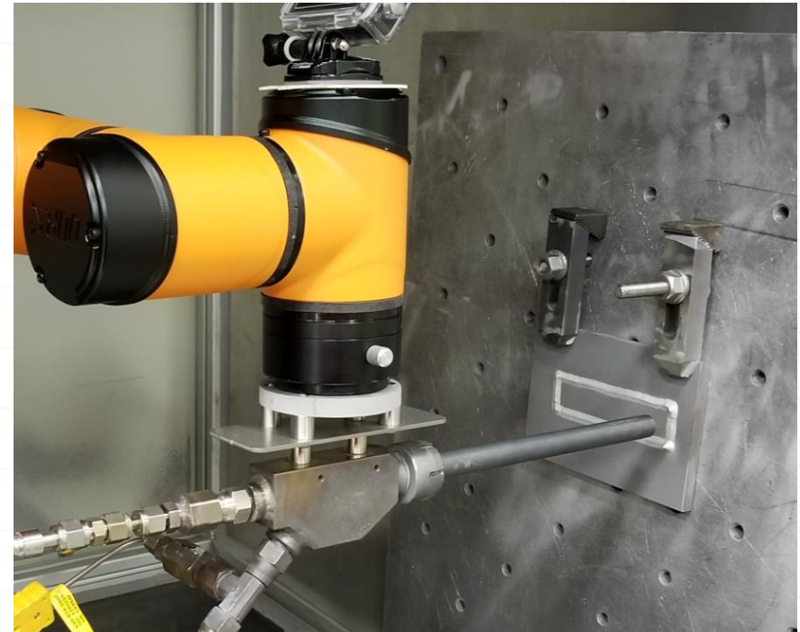
Previous robotic cold spray application completed by RTT
