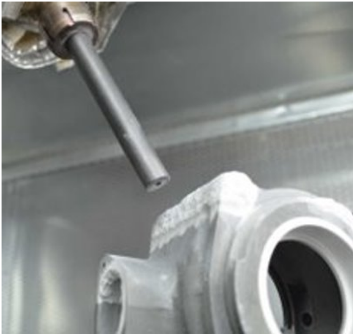
Cold spray application
