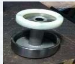
F-100 HPT Case Install/Lift Fixture
