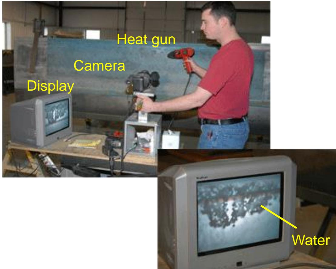
Thermographic inspection of CH-47 Main Rotor Blade using heat gun
