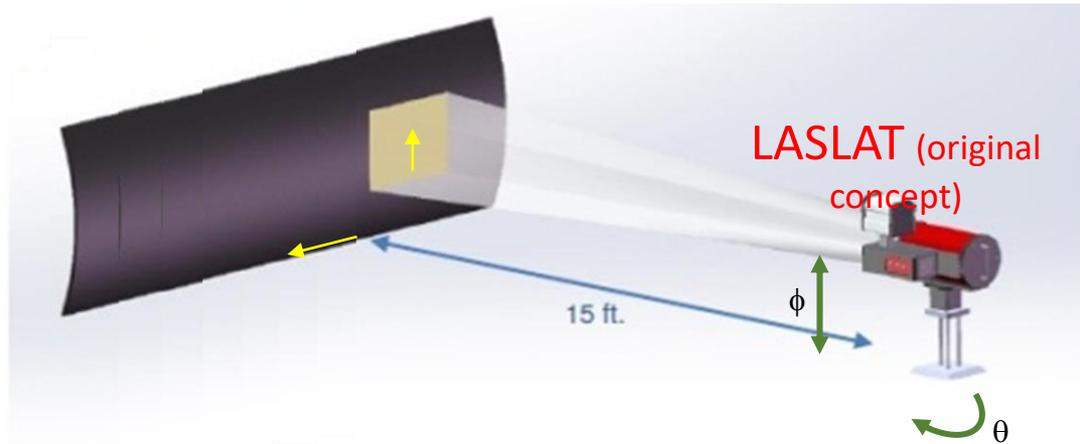
Objective: Provide the capabilities of flash thermography from a distance in a system optimized for NDI of large composite structures
