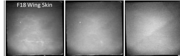
LASLAT signal processing outperforms existing NDI for detection of fluid ingress and impact damage.
