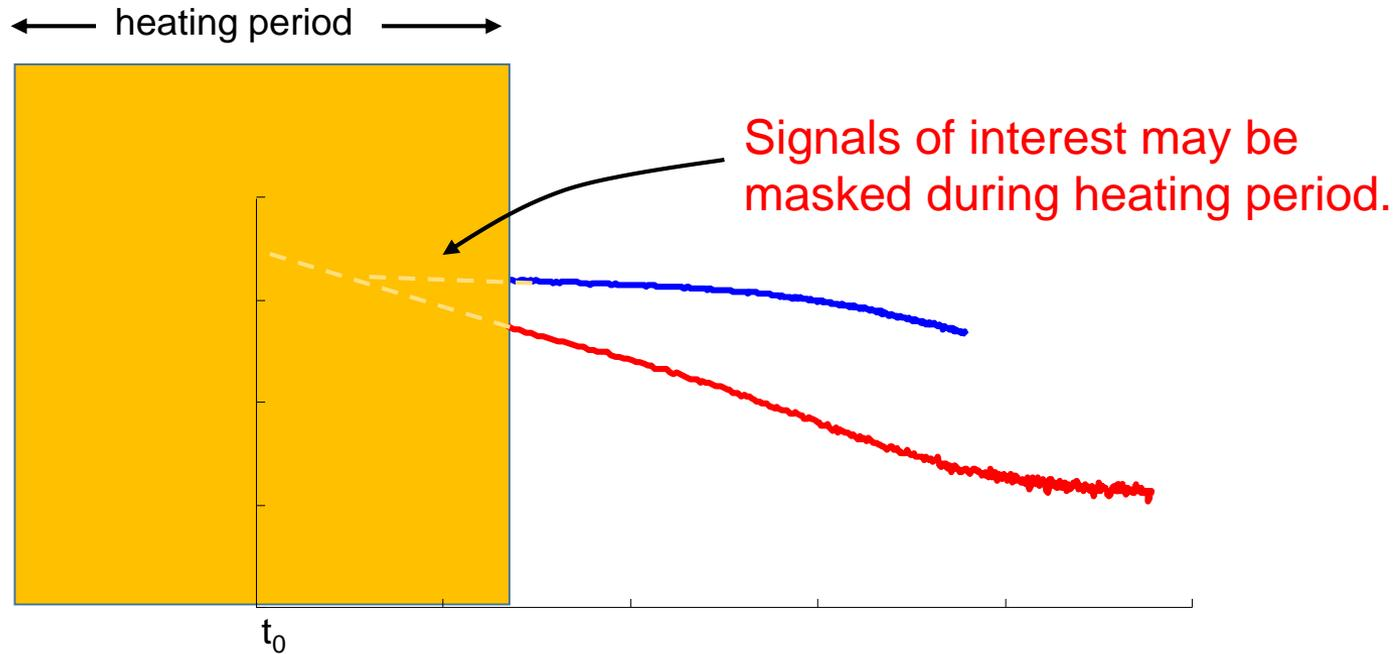
Heating and cooling occur simultaneously during extended heating
