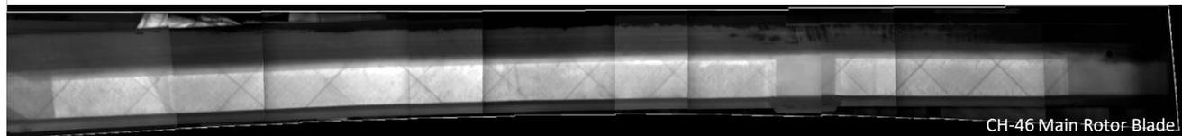
Optical correction over entire inspection field enables accurate defect sizing
