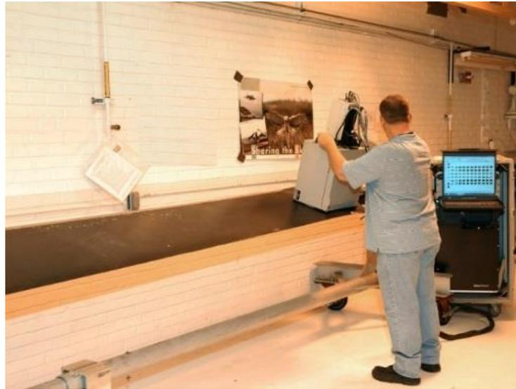
Current NDI of V-22 proprotor at FRC-E using TWI flash thermography system
