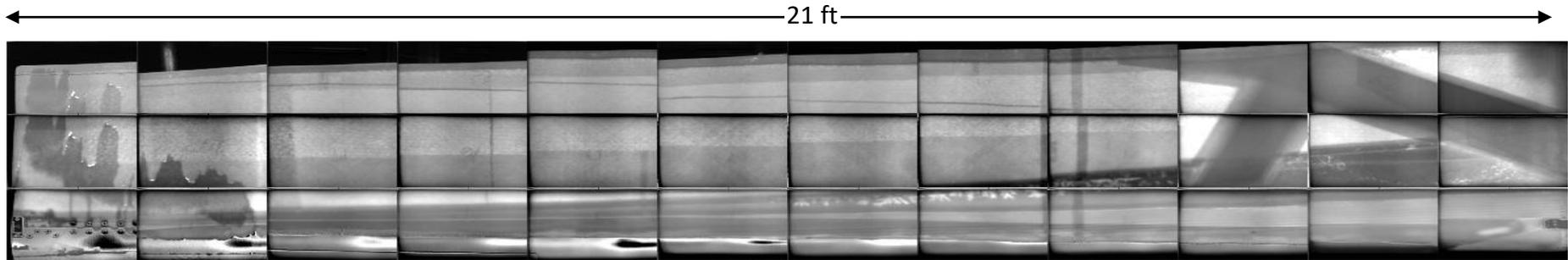
TSR processing of V-22 proprotor converts 36 shots into a single data set using TWI MOSAIQ software
