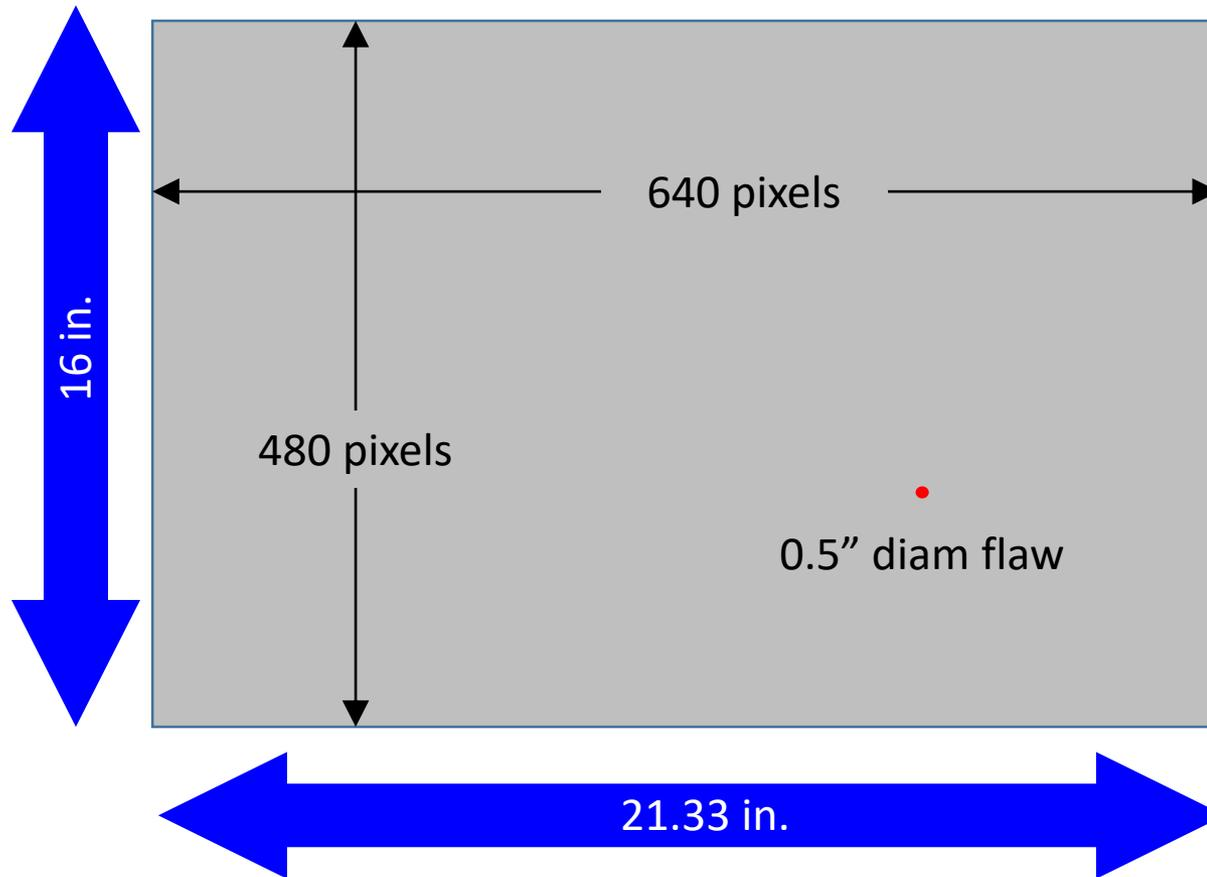
Maximum field of view to resolve a 0.5" flaw with a 640 x 480 pixel camera is 21" x 16"
