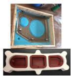
Casting in Urethane, Silicone with 3D Printed or Machined AL Molds
