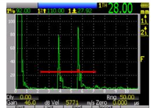
Straight beam A-scan image
