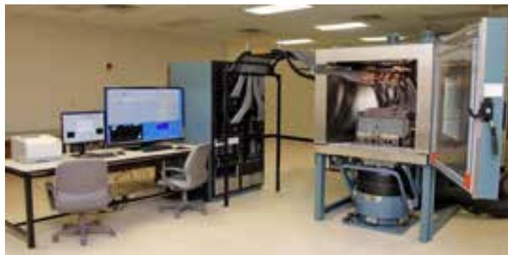
8000 test point Intermittent Fault Detection & Isolation System™ (IFDIS™) testing an F-16 AN/APG-68 Radar System Programmable Signal Processor (PSP)
