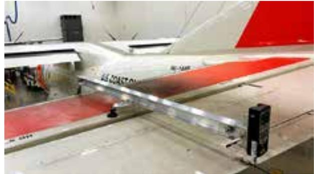
Figure 1: Portable "on-wing" prototype balance tool
