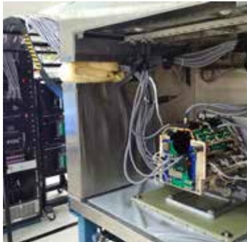
2800 test point Intermittent Fault Detection & Isolation System™ (IFDIS™) testing an F/A-18 Generator Converter Unit (GCU)
