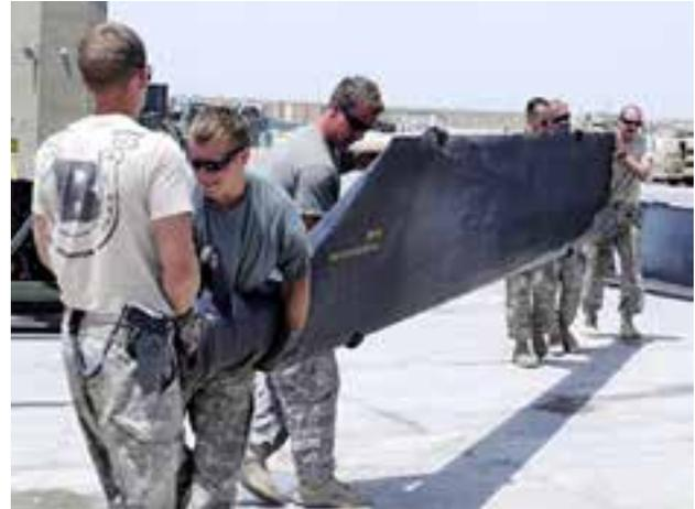
Supporting the full weight of the blade greatly increases the risk of injury and damage to the blade
