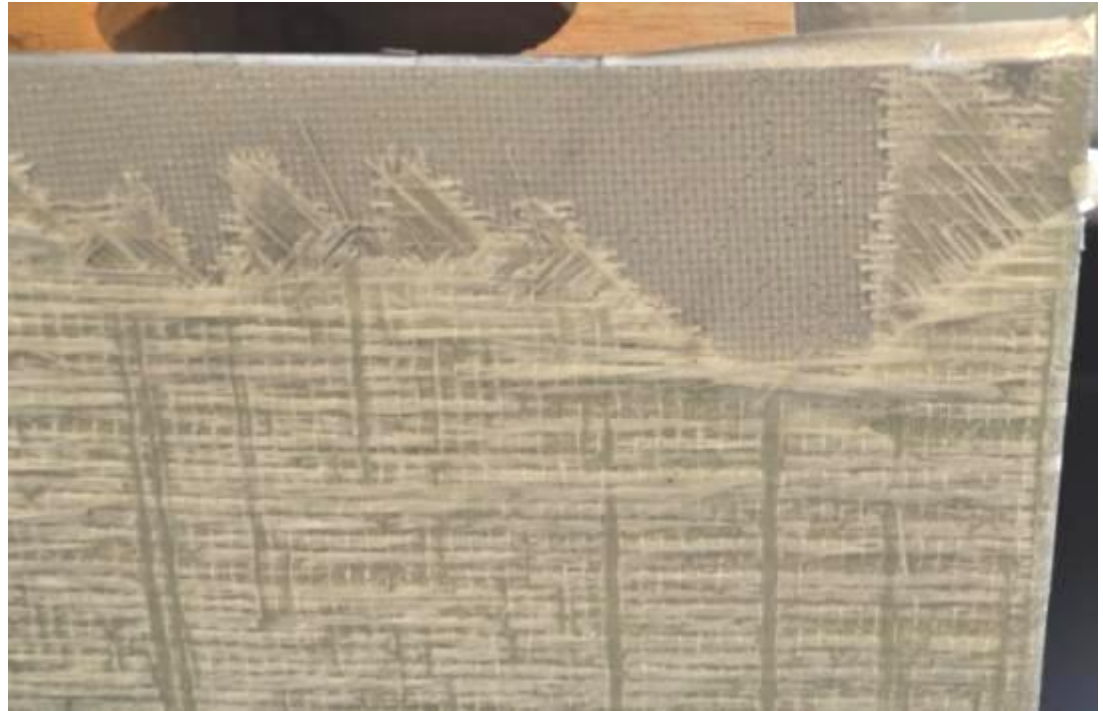
Lower Laminate Plies Adhered to Lower Plate
