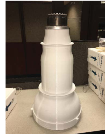
F108 fan shaft with and without 3D printed masking for thermal spray of dia “U”
