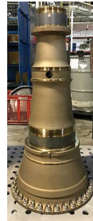
F108 fan shaft with and without 3D printed masking for thermal spray of dia “U”
