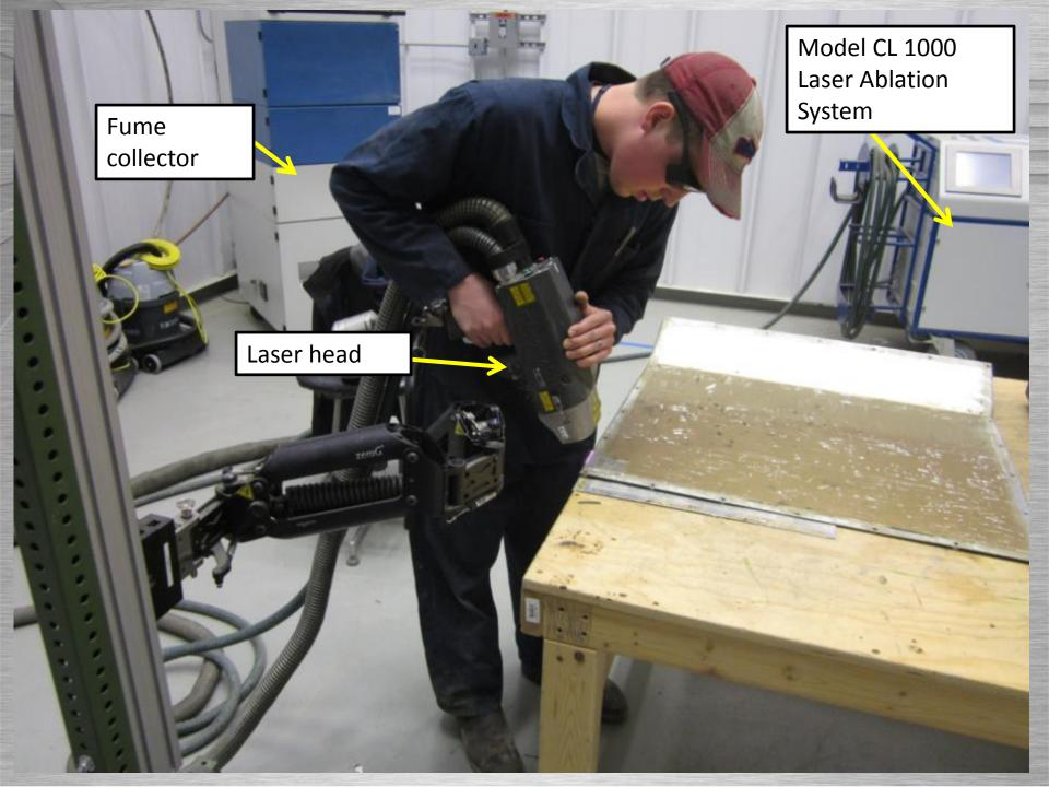
Laser end effector being attached to zeroG gimble
