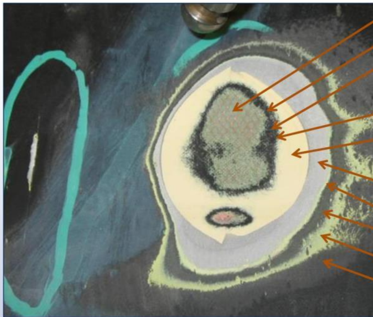
Coating Layers of V-22 prop rotor blade
