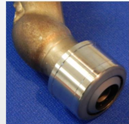
The same shroud after Laser Additive Repair and finish machine
