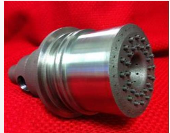
NASA SLM fuel injector for J-2X
