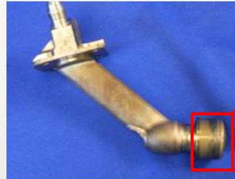
Fuel injector from gas turbine engine with worn air shroud
