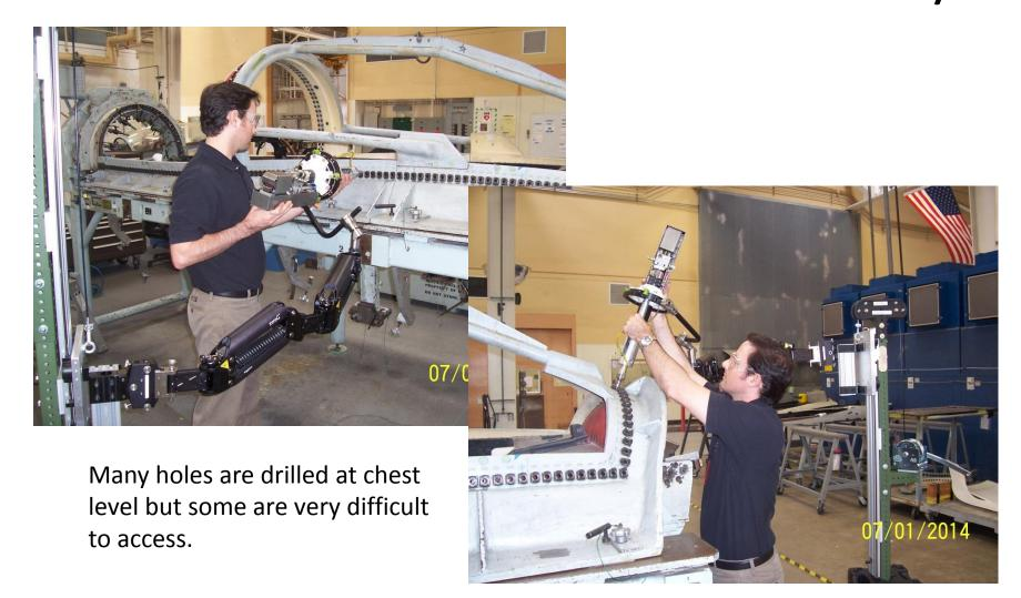
The drill needs to be rotated on it's horizontal axis to lock into the drilling fixture, and it must be held securely to the arm
