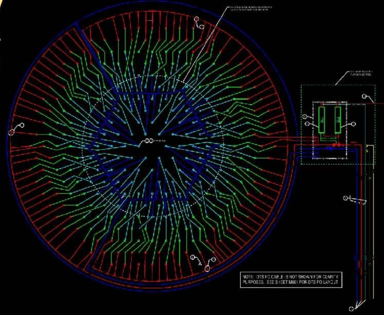
GEOTHERMAL BOREHOLE THERMAL ENERGY STORAGE (BTES) BOREFIELD LAYOUT
